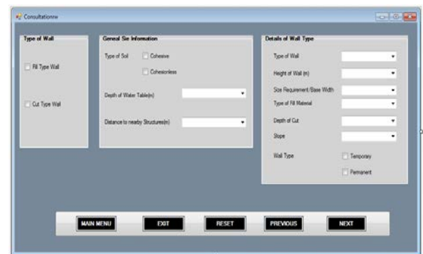
Fig.9.Consultation Module for Fill and Cut type walls
